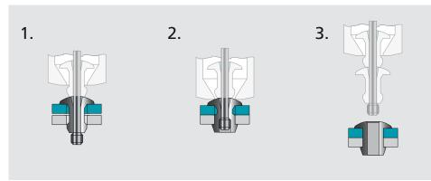
1. The mandrel with pre-loaded fastener is located in the hole.
